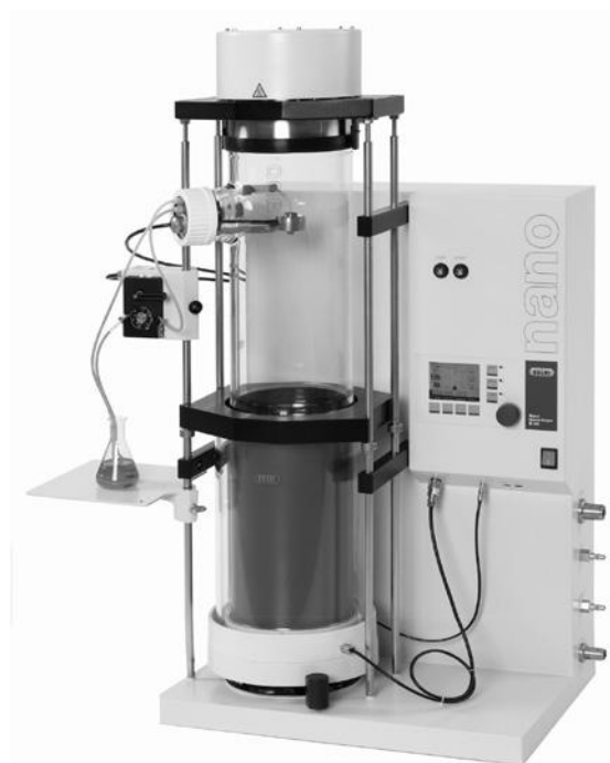
Fig. 29.11 • Nano spray-dryer. Courtesy of Buchi.
